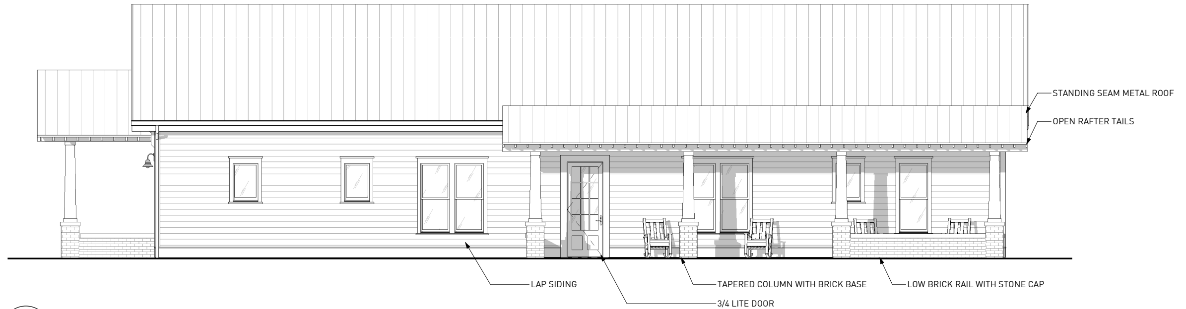
2 SIDE ELEVATION @ ROCKING CHAIR PORCH SD-3.1 1/8" = 1'-0"
